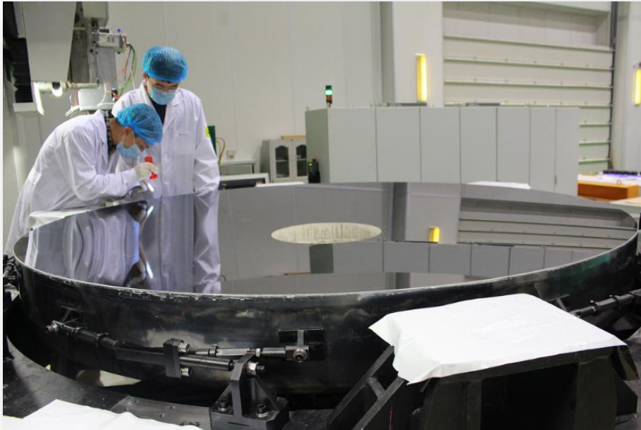
CIOMP's 2.2m SiC PM, 340kg (Areal Density: 89kg/m 2 )
